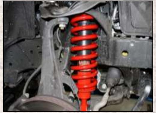
Terrafirma has teamed up with Pedders, World renowned Suspension manufacturers from Australia and now offers a range of Suspension upgrade kits for popular 4x4 pick-ups. Designed to provide a 40mm lift, improve the load carrying performance, ride comfort and appearance which allows for larger diameter tyres to be fitted. The kits are a complete engineered suspension solution for your pick up guaranteed to improve on road and off road handling and capability.
