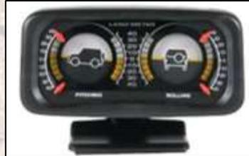
You can set your indicators to show the maximum angle the vehicle has achieved or more likely the point at which your nerves got the better of you! This inclinometer is mounted with double sided tape so no screws are required and includes wiring for back lighting.
